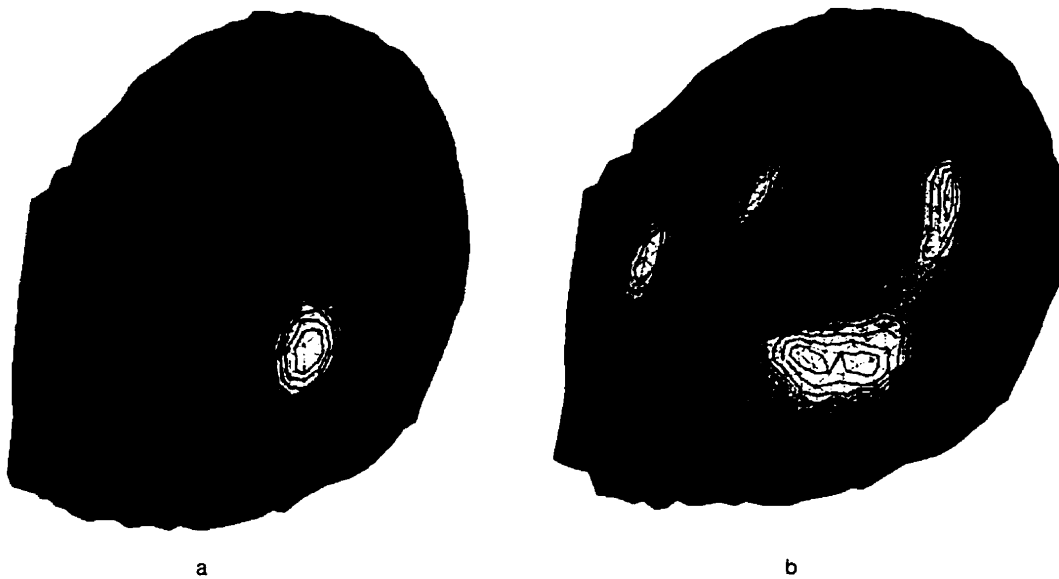
Figure 7.4: Visualisation of the displacement patterns along the x axis with the manubrium and the annular ligament clamped. The slice spacing is set to 2 and the nominal number of elements per diameter is 35. (a) Spline-interpolated tympanic membrane (same as in Figure 7.3a). (b) Manually segmented tympanic membrane.
