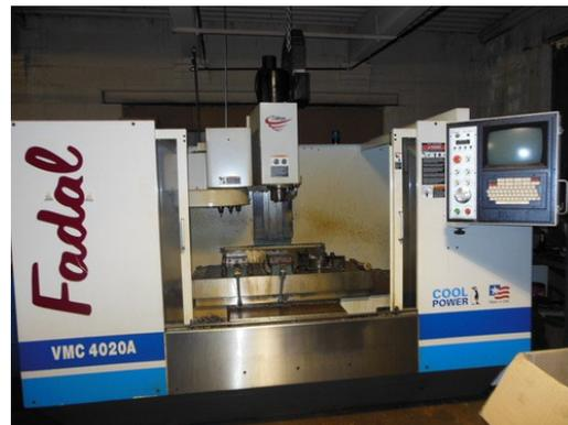
*Figure 4.14: CNC vertical milling machine with computer interface*
