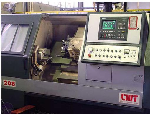
*Figure 4.13: CNC lathe machine with computer interface*
