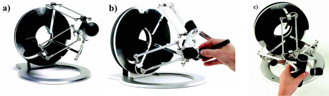
Figure 2.26: Force Dimension omega.x force-feedback haptic devices. a) omega.3 with 3 DOF in translations; b) omega.6 with 6 DOF: 3 translations and 3 rotations; c) omega.7 with 7 DOF: 3 translations, 3 rotations and 1 grasping (Force Dimension 2015).
