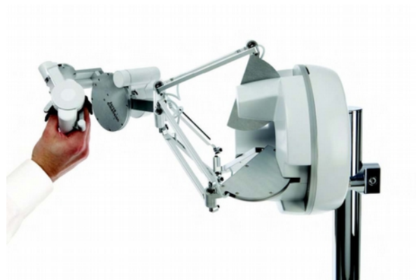
Figure 2.27: Force Dimension sigma.7 force-feedback haptic device with 7 DOF: 3 translations, 3 rotations and 1 grasping (Force Dimension 2015)
