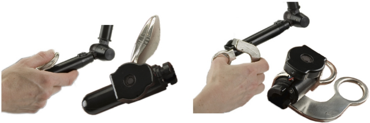
Figure 2.24: Thumb-pad (left) and scissors (right) snap-on end effectors for Phantom 6-DOF devices. These end effectors provide an additional degree of freedom in positional sensing (Sensable technologies 2007).
