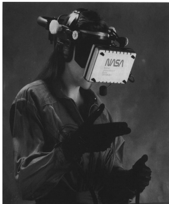
Figure 2.5: The Virtual Interactive Environment Workstation VIEW system, developed at the NASA Ames Research Center (Gigante 1993)
