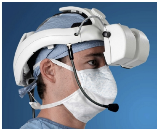
Figure 2.6: Opaque stereoscopic medical HMD from Viking systems (Keller et al. 2008)
