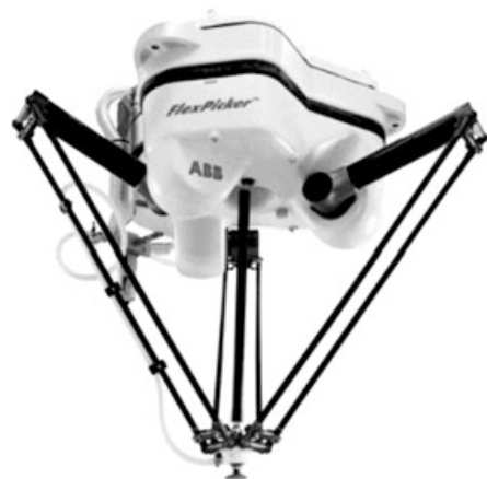
Figure 2.18: Type of delta robot introduced in production by ABB in 1999 under the name FlexPicker (Figure 7.1 in Lenarčič, Bajd, and Stanišić 2013, p. 240)
