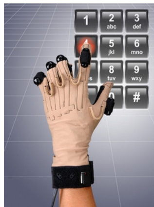
Figure 2.19: CyberTouch vibrotactile glove for generating touch sensations (CyberGlove Systems 2015)
